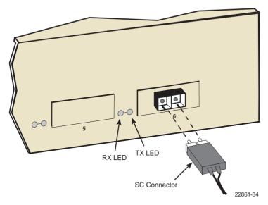
Figure 3-10 Fiber Optic Cable Connection
